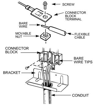
WARNING: CONNECTOR BLOCK IS APPROVED FOR COPPER WIRE CONNECTION ONLY. IF ALUMINUM WIRE IS USED, SEE NOTE BELOW.
